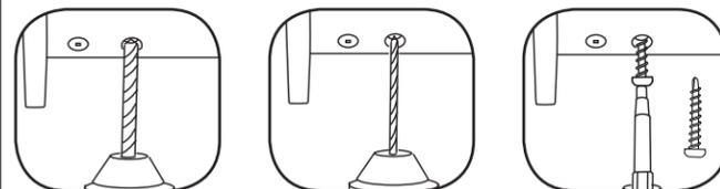
1. For each screw drill a counter sink the depth of the vinyl using a 9/32" bit.
